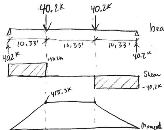
beam weight =  $55 \text{ plf} \times 18 \text{ ft} \approx 1 \text{ K}$ .
