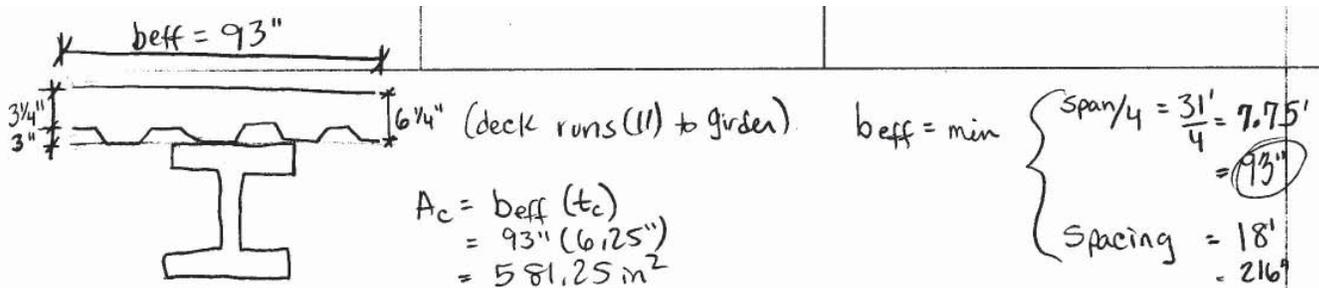
$$\begin{aligned} C_c &= 0.85 f'_c A_c \\ &= 0.85 (3 \text{ Ksi}) (581.25 \text{ in}^2) \\ &= 1482.2 \text{ K} = V_c' \end{aligned}$$
