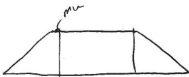
Max spacing @ mid section of beam = 3 feet.  $\rightarrow$  place 4 studs in mid section,
