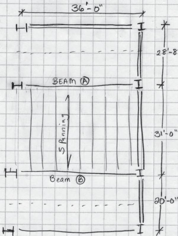
$W_{self} = \frac{370 \text{ lb}}{\text{ft}} \times \frac{1}{4 \text{ ft}} = 92.5 \text{ psf}$
